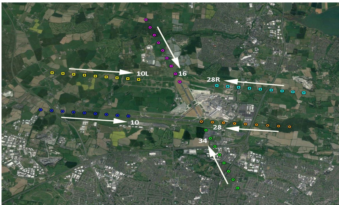
Figure 4: 2 mile approach lines to runways at Dublin Airport (at ¼ mile intervals) as assessed by SGHAT. Includes the proposed northern runways 10L and 28R.
