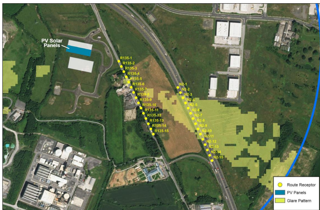
Figure 3: Route receptors identified within 1km of the proposed solar PV development that intersect with the predicted glare pattern.
